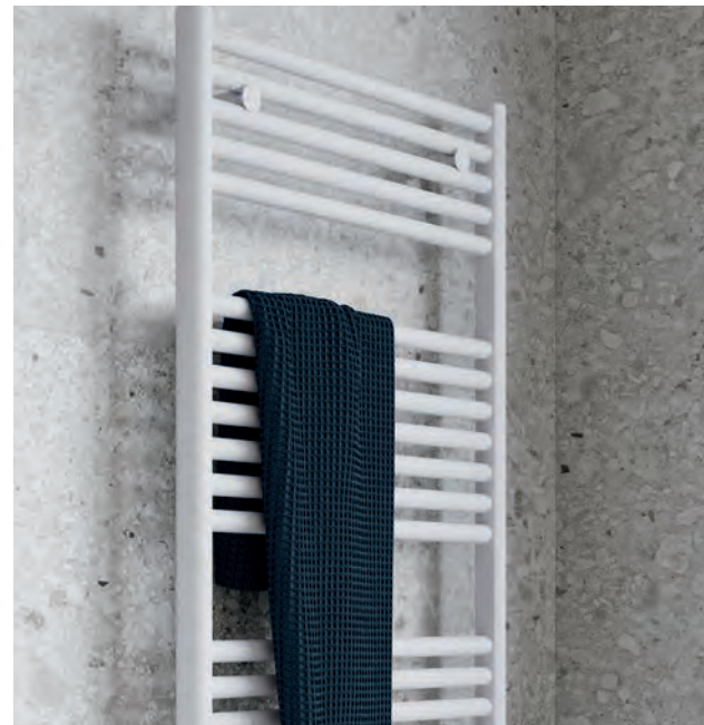
CC Tappings are 40mm less than the rail width and approx. 70mm from wall. We recommend using Hugo2 in a closed system incorporating an anti-corrosion inhibitor. All heat outputs based on Delta Δt 60°C.
