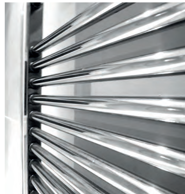
CC Tappings are 40mm less than the rail width and approx. 70mm from wall. We recommend using Hugo2 in a closed system incorporating an anti-corrosion inhibitor. All heat outputs based on Delta Δt 60°C.
